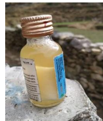
Image of vial with light brown colour indicates that water is fit for drinking.
