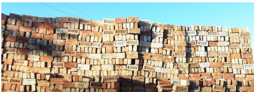
Figure 27: Stacking of fired bricks.
