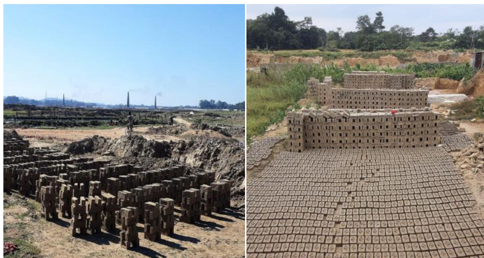
Figure 23: Different stacking patterns during brick drying phase (left and right).
