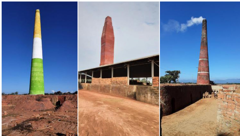
Figure 13: Different kilns from the demand centres. Semi-covered kiln design such as the one observed in Silchar (centre) allows for brick production during adverse weather conditions
