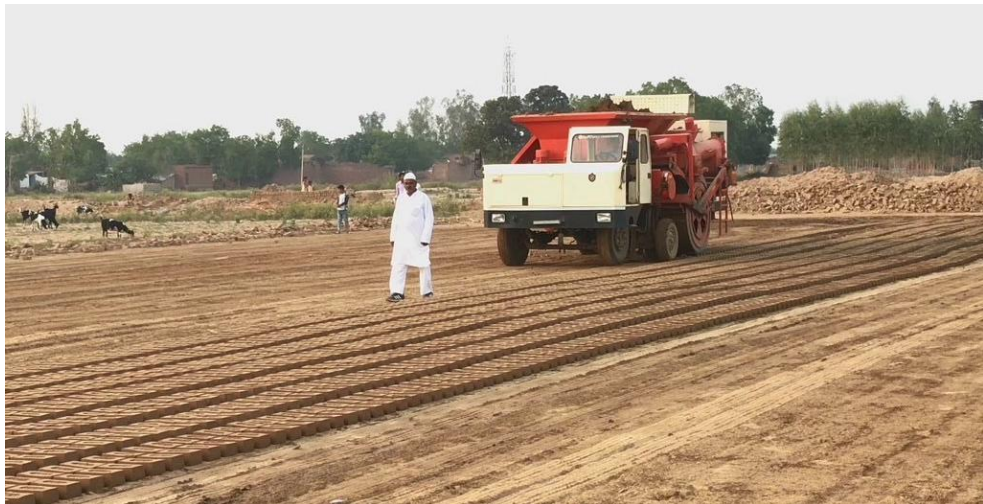
Figure 21: Automatic movable brick extrusion machine
