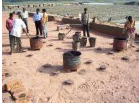
Figure 35: Firing of bricks in high draught Zigzag kiln
