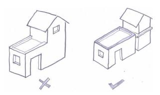
This has been demonstrated in the community building in Kamad village. A connecting corridor was provided between the single storied and double storied parts of the building. The corridor is connected with the ground floor section of the building and is simply supported on brackets provided in the double-storied section. This will ensure that torsion caused by asymmetric constraint to lateral forces will not arise in case of earthquake.
