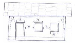
All openings should be at a distance of at least 450mm from the inside corner of rooms and must be at least 600mm apart. The cumulative width of openings should not be more than 50% of the total length of the unsupported wall.
