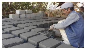
Concrete blocks are large sized masonry units made by compacting a well graded concrete mix. Since they can be produced easily using simple moulds. thev are already being produced by house-builders in the mountain region. Although it is an appropriate material for localized production, there is no awareness of its basic requirements for quality- namely adequate the correct mix and
