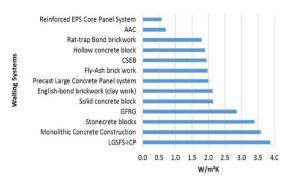
**Figure 19**: Thermal performance of selected walling systems
