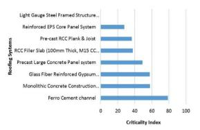
Figure 16: Critical resource use in selected roofing systems
