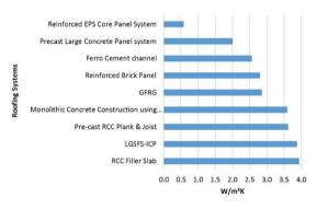
Figure 20: Thermal performance of selected roofing systems
