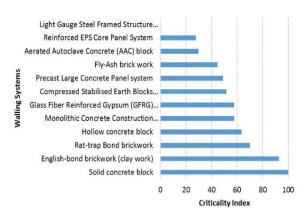
Figure 15: Critical resource use in selected walling systems
