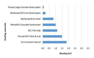
**Figure 24:** Job creating potential of selected roofing systems
