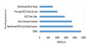
Figure 22: Construction cost of selected roofing systems
