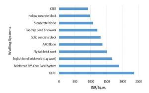
Figure 21: Construction cost of selected walling systems
