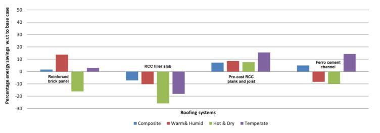
Figure 26: Impact of roofing systems on cooling energy consumption w.r.t to the base case
