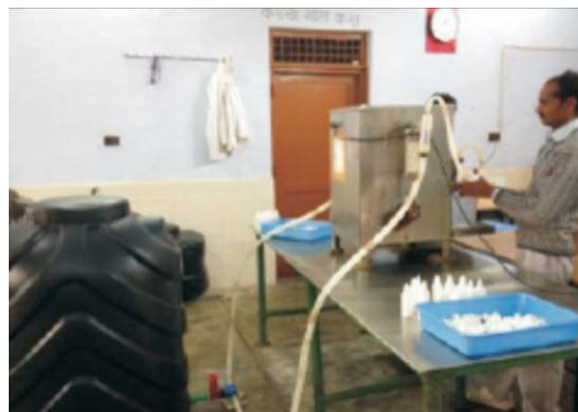
Figure 2-13: Bottling of Chlorine at the new Production plant
