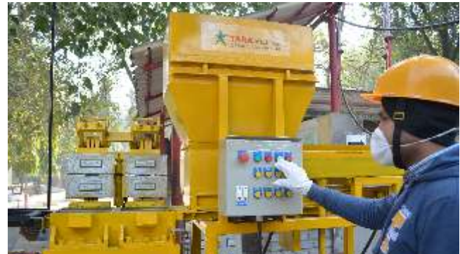
Fly ash Bricks Machine being operated to produce energy efficient bricks substituting clay bricks.
