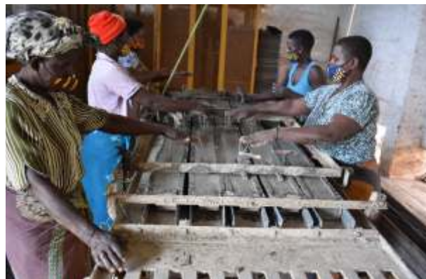
Training on RCC door frames at Eco-Matters, Lilongwe, Malawi
